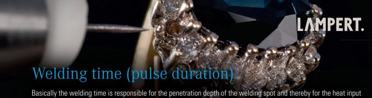
Basically the welding time is responsible for the penetration depth of the welding spot and thereby for the heat input into the workpiece. Hence, it must be observed when small material thickness and heat sensitive materials like gemstones are involved. Especially the new PUK 4 and PUK 5 series provide extremely short welding times starting from 0.5 ms. With this, the work on sensitive pieces and directly next to gemstones or sensitive materials like even plastic is feasible without any problem.
